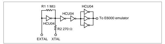
Figure 9 Oscillator Circuit
